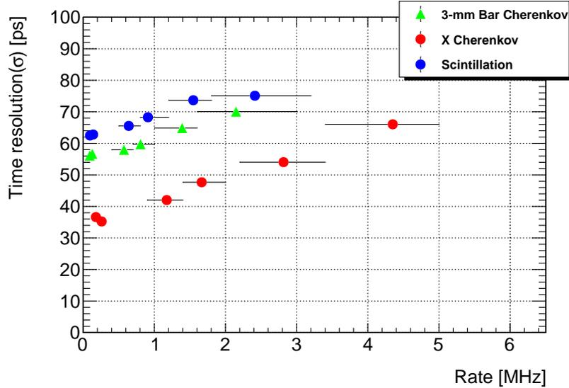
Figure 3: Counting rate dependences of time resolutions by the HUL module. All detector achieved time resolution of better than 80 ps (rms) at the counting rate of 2-3 MHz.
