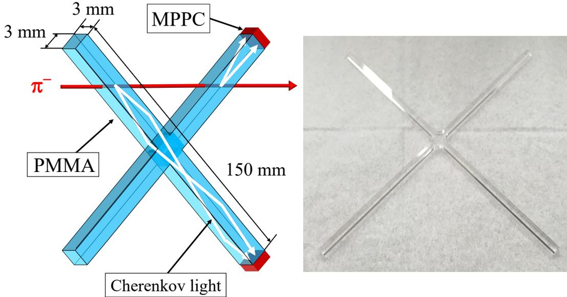
Figure 1: X-type Cherenkov detector. A cross-shape radiator which is cut out an X-type acrylic from an acrylic plate.
