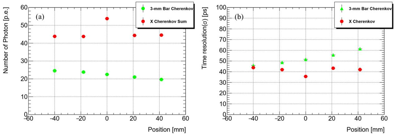
Figure 2: The position dependence of the photoelectron(a) and time resolution(b).
